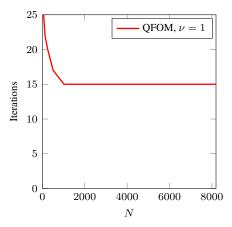
Fig. 5.3. Number of multigrid iterations needed to reduce the initial residual by  $10^{-12}$  as a function of N.
